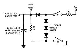
Figure 3. Load Test Circuit for TRI-STATE Outputs
